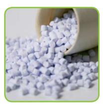
La Chira produce per estrusione granuli termoplastici in polipropilene (compounds).
